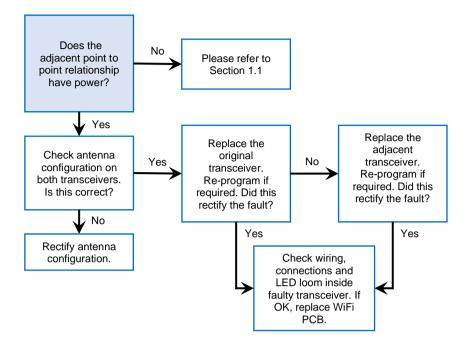
Section 1.1 - Transceiver - No power/lights, Flow Chart
