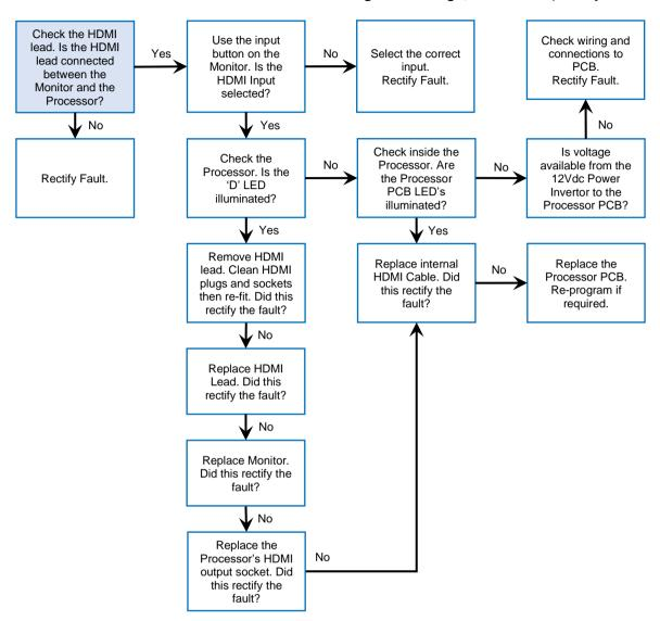
Section 1.10 - M3 Transceiver - No data input/output, Flow Charts (M3L System Only)
