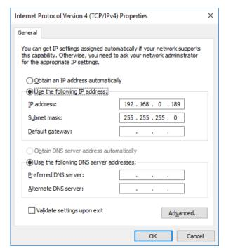
An IPv4 IP Address is made up of 4 Octets. The first, second and third Octet must be identical for connectivity across all paired units. The fourth Octet must be unique to avoid conflicting IP Addresses.
