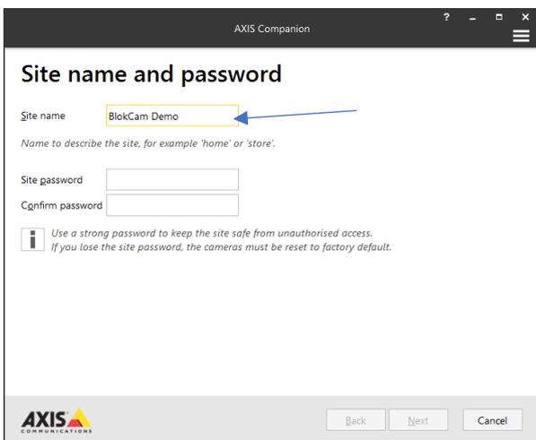
4. Obtain the Site password from an authorised BlokCam® dealer. Do not create a password. Creating a password will lead to system failure.
